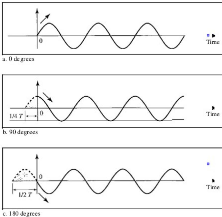
Phase is measured in degrees or radians [ $360^\circ$  is  $2\pi$  rad;  $1^\circ$  is  $2\pi/360$  rad, and 1 rad is  $360/(2\pi)$ ]. A phase shift of  $360^\circ$  corresponds to a shift of a complete period; a phase shift of  $180^\circ$  corresponds to a shift of one-half of a period; and a phase shift of  $90^\circ$  corresponds to a shift of one-quarter of a period (see Figure 3.5).
