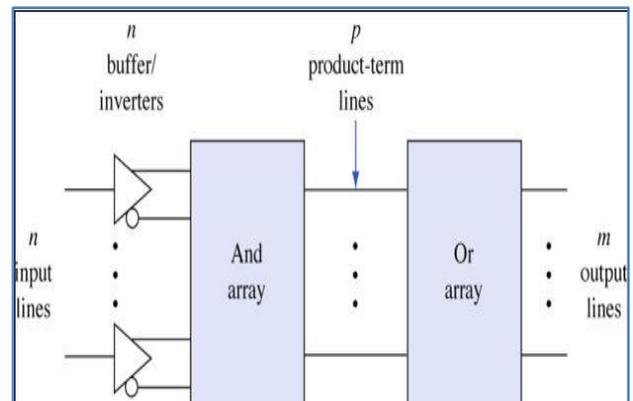
One of the simplest programming technologies is to use fuses. In the original state of the device, all the fuses are intact. Programming the device involves blowing those fuses along the paths that must be removed in order to obtain the particular configuration of the desired logic function.
