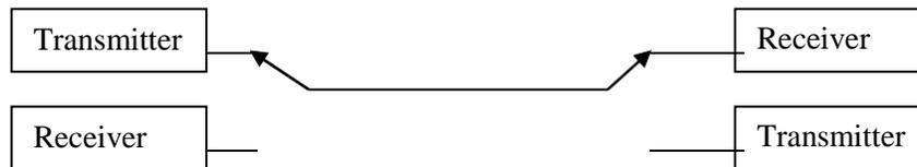
**3. Full duplex communication link:** If the data is transmitted in both ways at the same time, it is a full duplex i.e. transmission and reception can proceed simultaneously. This communication link requires two wires for data, one for transmission and one for reception.
