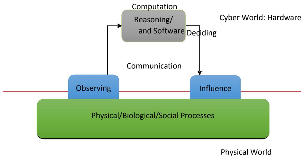
Figure 1: A Cyber-Physical System uses feedback to influence the dynamics of a Physical Process by taking decisions in the Cyber-World.
