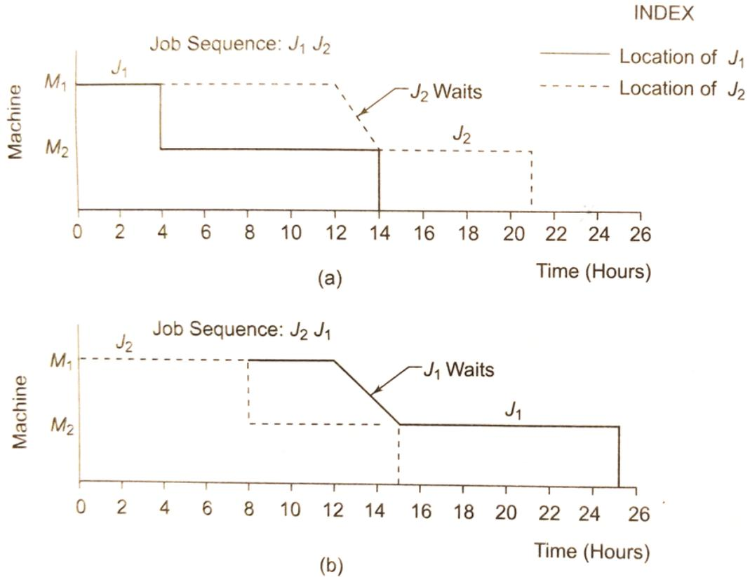
For processing the two jobs, two orders are possible  $J_1$ - $J_2$  and  $J_2$ - $J_1$ . Both these alternatives are evaluated in the above figure. The first part of the figure depicts the job sequences  $J_1$ - $J_2$ , according to which the two jobs can be completed in 21 hours. The other sequence  $J_2$ - $J_1$  depicts that the two jobs would take 25 hours to finish.
