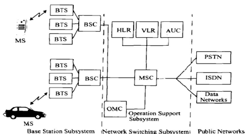
Fig2: GSM system Architecture
