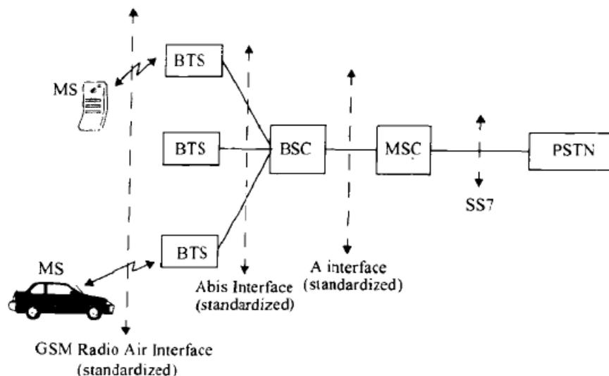
Fig 3 The various interfaces used in GSM
