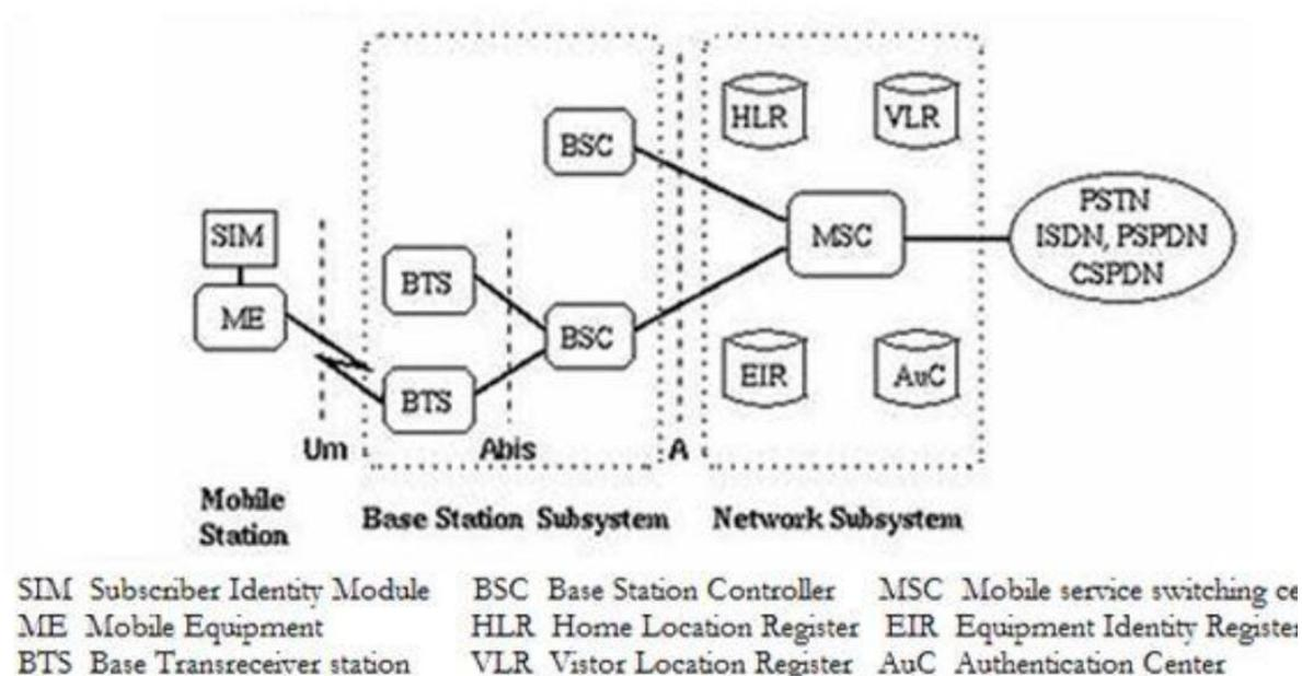
The GSM network architecture consists of three major subsystems:
