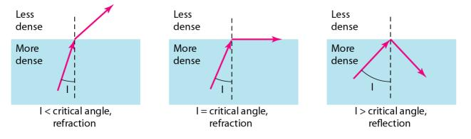
As the figure shows, if the angle of incidence I (the angle the ray makes with the line perpendicular to the interface between the two substances) is less than the critical angle(the angle of incidence which provides an angle of refraction of 90 degree), the ray refracts
