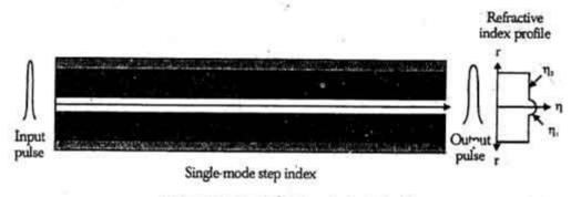
Light propagation in single mode step index fiber
