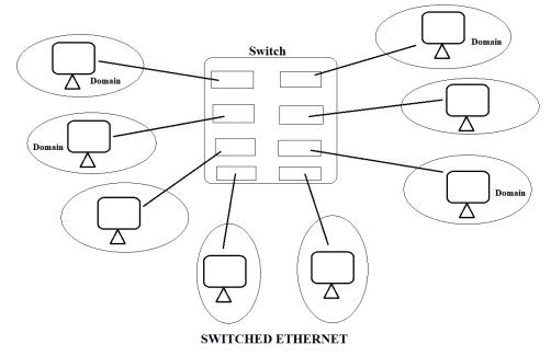
In such a case, the bandwidth is shared only between the station and the switch. The collision domain is also divided into N domains.
