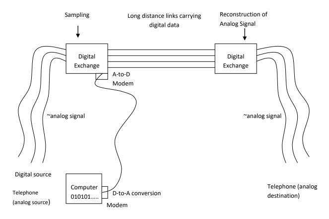
Telephone signal which is analog up to exchange is sampled at the exchange by taking 5 samples per second. Each sample value is represented by b bits/sample. So s \* b bits/second are generated.
