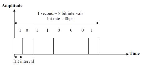
The bit interval is the time required to send one single bit. The bit rate is the number of bit interval per second. This mean that the bit rate is the number of bits send in one second, usually expressed in bits per second (bps) as shown in Fig1. A digital signal can be considered as a signal with an infinite number of frequencies and transmission of digital requires a low-pass channel as shown in Fig2. On the other hand, transmission of analog signal requires band-pass channel shown in Fig. 3.
