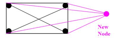
Fig(b) Adding a new node in Mesh Topology
