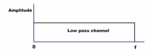
Fig1. Low pass channel required for Digital signal
