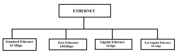
Fig(a) Ethernet Evolution through four Generations
