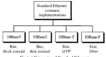
Fig (c) Categories of Standard Ethernet
