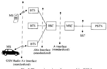
Fig 3 The various interfaces used in GSM
