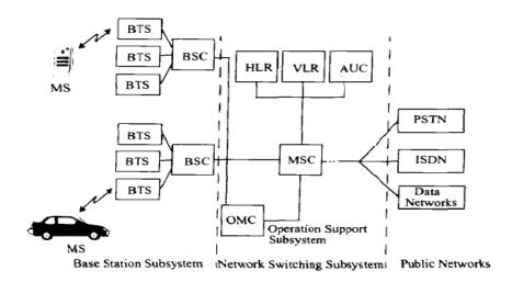
Fig2: GSM system Architecture
